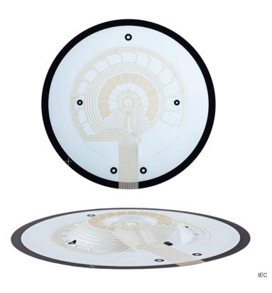
NOTE 1 The top image shows a 2D substrate and ink stack after printing and cure.
